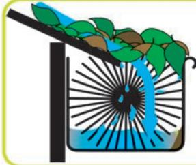
Ideal for collecting water for a tank, pool or spa. Less dust and debris is stirred up when water enters the gutter. brushguard allows the water to run down the bristles and "soft fall" into the gutters.
