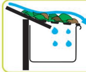
Leaves can form a seal over single plane gutter systems making it less effective. Water flows over the leaves and off the edge of the gutter.
