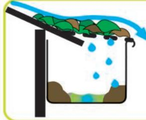
Any water that does get through traditional gutter protection, stirs up the debris creating a sludge which increasing the chance of contaminated water & rusting gutters.
